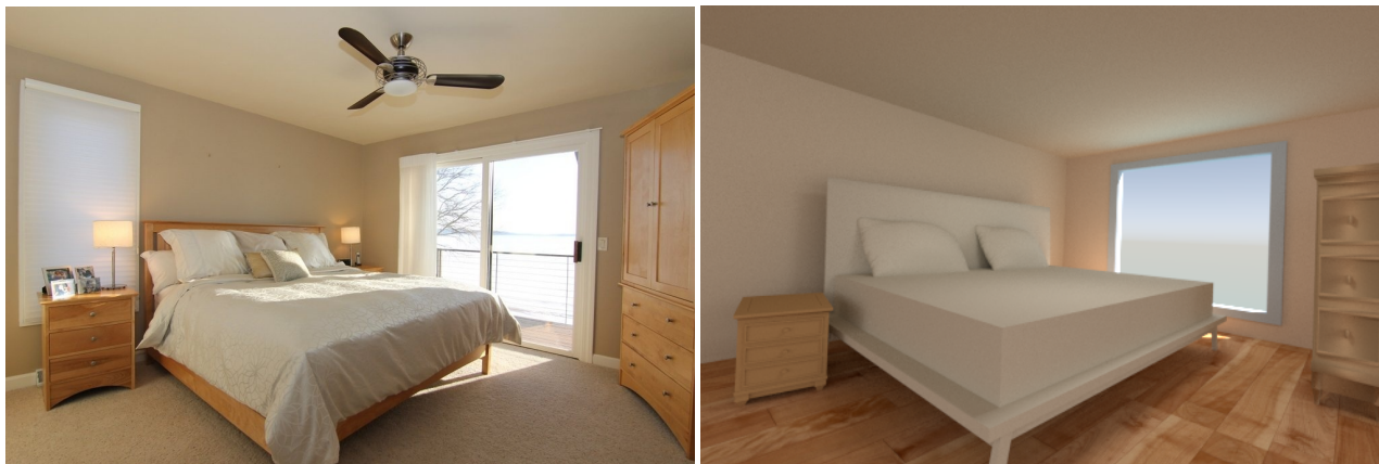
Figure 1: IM2CAD takes a single photo of a real scene (left), and automatically reconstructs its 3D CAD model (right).
